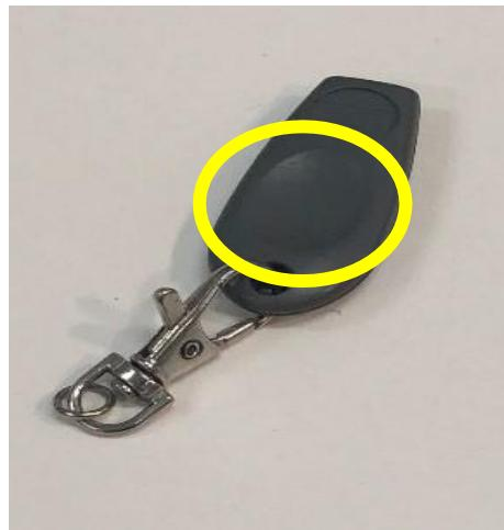
Hold the oval key tag perpendicular to the reader and at the centre of the reader as shown below, wait for the beep and colour on the reader to change from red to green.
